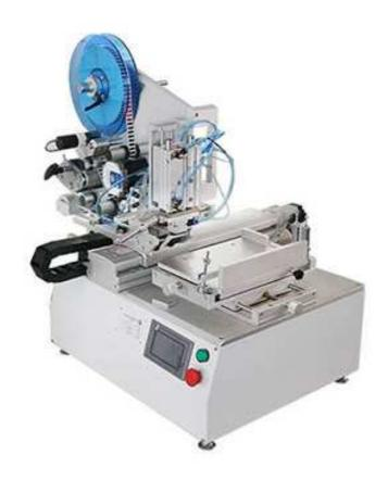
HL-T-101 Applicable to all kinds of precision products on the plane labeling change the label suction head to meet the small size labeling. Such as the diameter of 5mm tag labeling.
