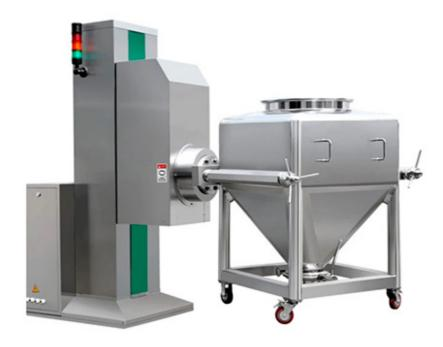
HTD Series Column post bin blender is mainly used in blending of solid particle and dust powder materials in pharmaceutical industry. With features of being easy in loading and discharging and having good blending effects it is also widely used in food and chemical industries.
