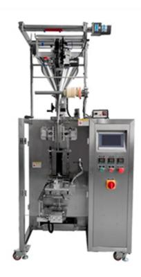
The machine is suitable for fully automatic round corner bag packaging of powder materials in food, pharmaceutical, and other industries, for example, coffee powder, match powder, milk powder, protein powder, herbs powder, spice powder, etc. This reciprocating powder packaging machine uses special-shaped punching, sealing, and cutting, to improve the sealing appearance of finished bags.
