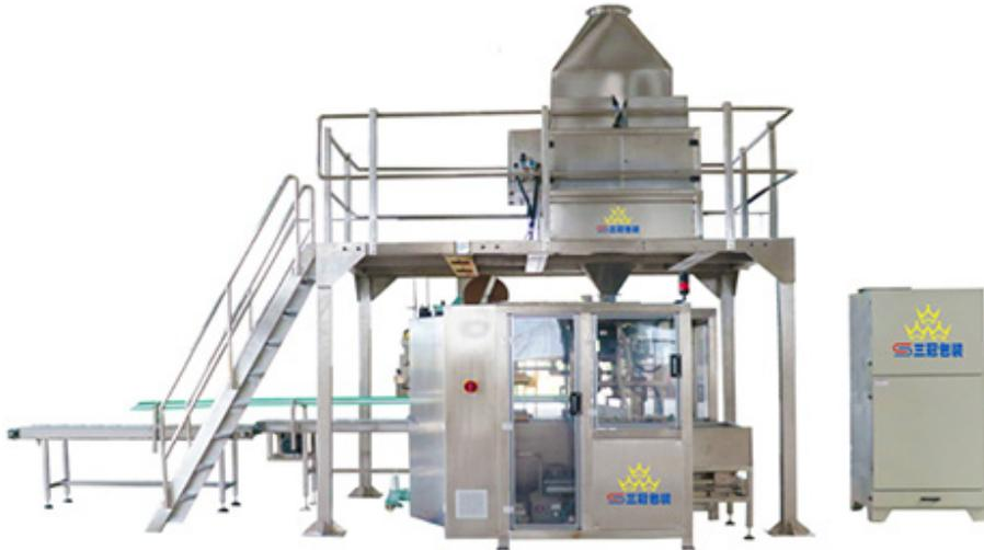
SGJ-ZDF Automatic Powder Bagging Machine Line is the newest developed machine model which focuses on automatic powder material weighing, filling, bag feeding, clamping, conveying & sewing, finished products take-off, shaping conveying, robot palletizing & pallet bank system. The powder bagging machine line is now widely applied in packing wheat flour & tapioca starch. The bagging machine line is suitable for packing powder material within 60 meshes in size.
