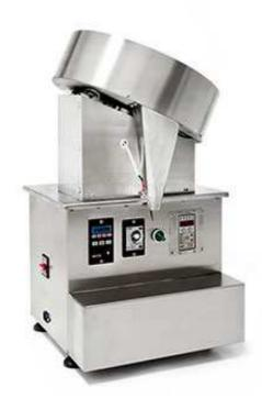
Application: widely used for counting and filling of capsules, pill, tablets.
