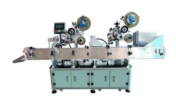
T402B Double Heads is suitable for labeling the non-free standing round bottle while conveying. It is automatic feeding and automatic labeling, adopting horizontal conveying mode, It will increase the smoothness of conveying and improve the labeling precision.
