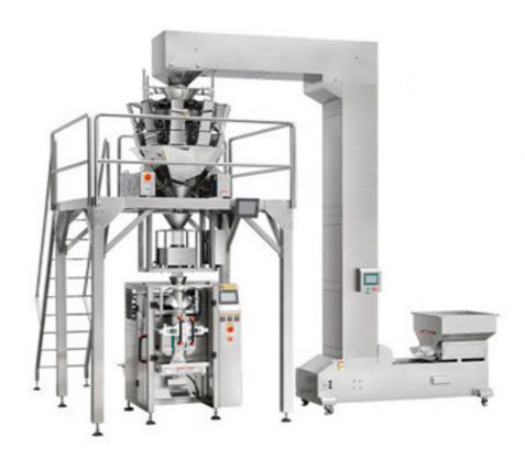
The DC-890B high-speed, turn-up collar, back-seal packaging machine uses toothed cutting and back sealing. Coupled with a metering device, this machine can automatically complete the entire process of feeding, bag making, filling, bag sealing, date printing, inflation (exhaust), and finished product output.
