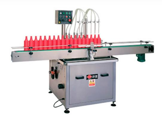
AF-80 liquid filling equipment common application is for above 60mL low viscosity liquid products such as collagen healthy drinks, mouthwash and etc. In order to meet customer's various requirements, minor modification for the equipment is also applicable.
