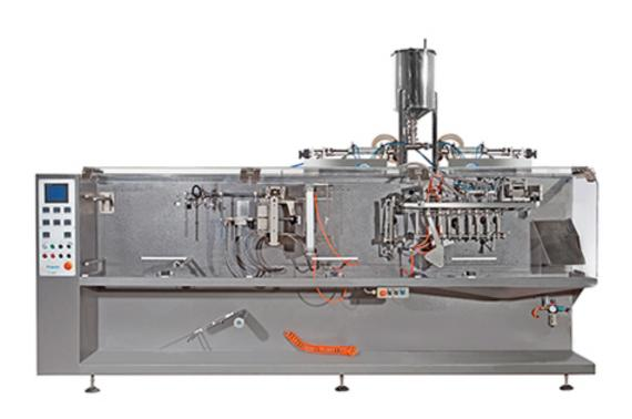
XT-180 is automatic horizontal film packing machine which is designed for bag middle size and small size and dual filling function. It is widely used in the packing fields of food, pharmaceuticals, house chemicals, cosmetics, etc. And it is suitable for powder, granule product and liquid product, etc. with different products, use different fillers. it is your wise choice for three-side, four-side seal and two or more-link bag function.
