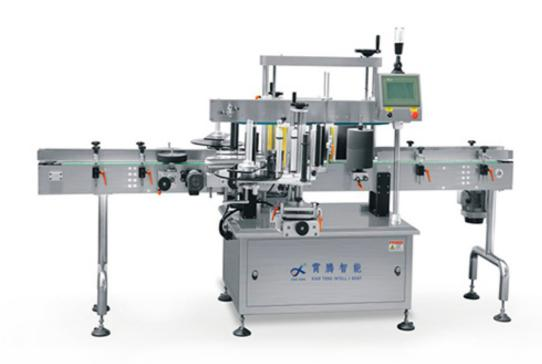
Applicable to pharmaceutical, food, daily chemical and other light industry round, square and flat bottles single side labeling, one machine suitable for square bottle, flat bottle and round bottle, can be used alone or connect with the production line.
