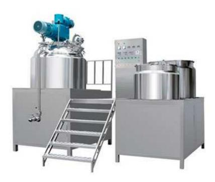
Vacuum homogeneous emulsifying machine is a set of mixing, dispersion, emulsification and homogenization, powder absorbing functions in one integrated system, a control system, but also with the peripheral oil, water tanks, the use of vacuum, heating / cooling system. Is a special equipment for producing medicinal ointment, cream, lotion and other high-grade.
