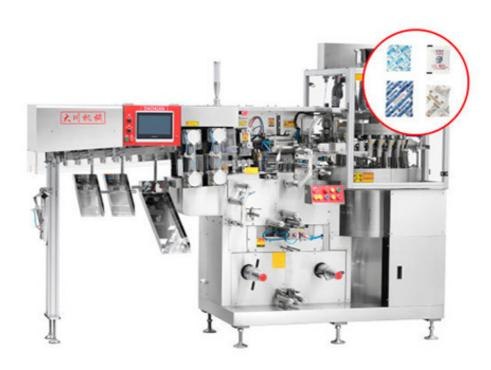
The rotary system automatically forms bags, fills them, seals the edges, and counts them horizontally, with a machine speed of 300-460 bags per minute. The bags produced by the machine have aesthetically pleasing and tight seals.
