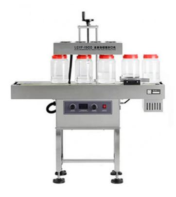
LGYF-1900 Continuous induction foil sealer uses electromagnetic induction sealing technology to seal the bottle, the technology has fast sealing speed, no contact in the whole process, and the product has good sealing performance.
