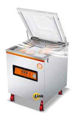
This vacuum packaging machine has automatic processing functions such as vacuuming, sealing, and cooling. It is suitable for vacuum packaging in food, medicine, aquatic products, chemicals, electronics and other industries. It can prevent product oxidation, mildew, corrosion, moisture, maintain quality and freshness, and extend storage period.
