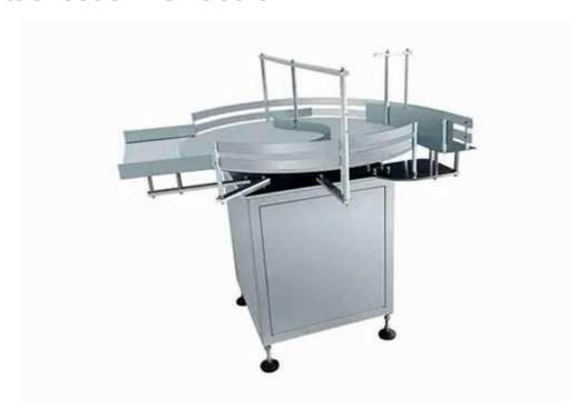
The device is to manually put the messy bottles onto the disc, and through the automatic rotation of the disc, the bottles are fed to the conveying line of the next process, and it has the buffering function. The whole machine is made of 304 stainless steel, meeting the requirements of GMP specification
