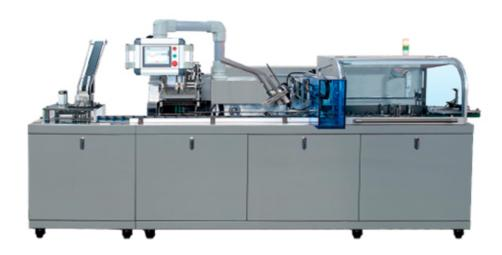
CT-100 is an intermittent motion medium-high speed cartoning machine. It is suitable for cartoning of tubes, bottles, bars as well as blister packs.
