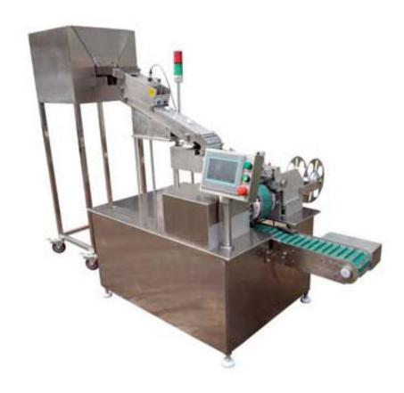
YJB-40 tablet wrapping machine is designed for wrapping in one roll with several pieces of tablets by aluminum foil and paper laminated material. YJB-40 tablet wrapping machine is controlled by PLC and it is very stable and reliable, and easy to operate and maintain.
