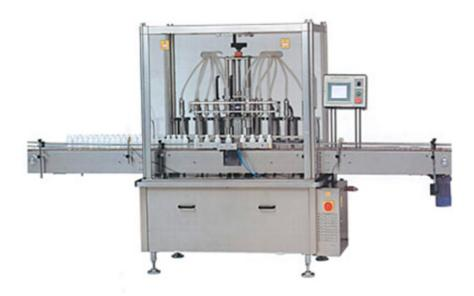
6 nozzles fill simultaneously. Number of nozzles can be increased according to requirement.
