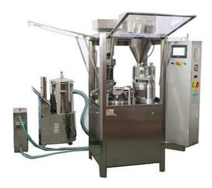
This machine is an intermittent motion and hole plate type filling fully automatic capsule filling equipment.
