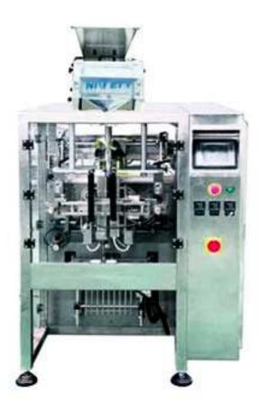
The single-file equipment counts and fills capsules, soft gels, normal tablets, special shape tablets, coating tablets, pills and most solid granules in small bags. Counts by infrared and sensor that doesn't wear or break the product and is compatible with all kinds of materials. Can accomplish bag forming, counting, filling, bag sealing and printing at the same time.
