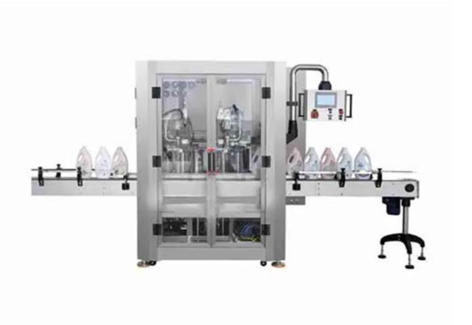
The machine is suitable for filling pastes and liquids. The filling piston dosing cylinder is driven by a servo motor; the filling volume can be controlled by adjusting the stroke position of the servo motor.
