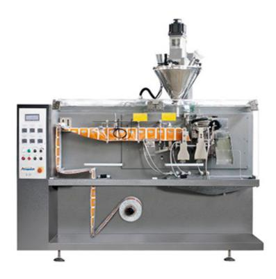
XT-110 automatic horizontal packing machine from Roll of film, machine is widely used in the packing fields of food, pharmaceuticals, house chemicals, cosmetics, etc. And it is suitable for powder, granule product and liquid product, etc. uses different fillers for different products. XT-110 series have simple design,100% pouch opening rate, it is your wise choice for three-side, four-side seal and two or multi-link sachet packing.
