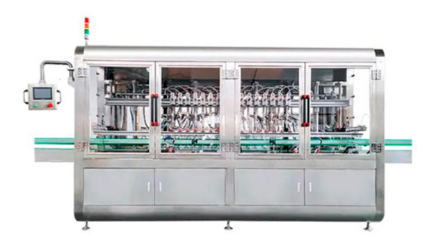
The NP-OF Inline overflow liquid filling machine is expertly crafted for accurately dispensing foamy liquids and products that demand uniform fill levels. Perfect for glass bottles or robust, solid containers, this filler delivers precise filling with a focus on visual quality.
