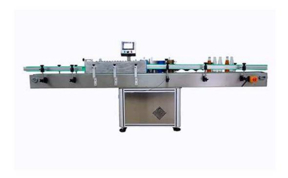
It's one of paste labeling machine, be used to paste label on all kinds of round bottle, to subdividing paper, coating paste labeling, label covering automatically.
