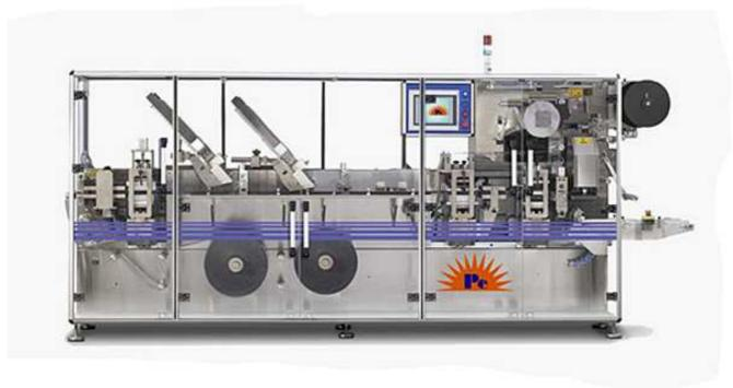
The PEW-RP-MACAV1 is suitable to Blister Pack 1ml, 2ml and 5ml Ampoules. The machine has a unique cantilever design with frontal format part accessibility in a modular balcony type construction. The basic machine comprises of mild steel chassis with SS 304 frames welded and bolted to form a rigid frame device structure on which various modular stations are mounted in balcony design (from GMP compliance and pharmaceutical sanitation standards).
