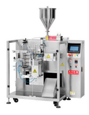
The DC-780M mini (low-speed) form-fill-seal packaging machine can be equipped with electronic scales, liquid metering pumps, servo screws, bowl-type feeding systems, etc., according to the material. It is suitable for fully automatic form-fill-seal packaging of liquids, sauces, powders, granules, and blocky materials.
