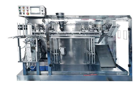
Compare to the rotary type premade pouch packing machine, the price of horizontal doypack machine is relatively more economical, but do not as versatile and multifunctional as rotary doypack machine.
