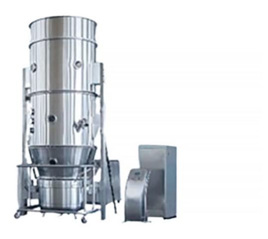
The powder granule in fluid bed appears in the state of fluidization. It is preheated and mixed with clean and heated air. At the same time the solution of adhesive is sprayed into the container. It makes the particles become granulating that contains adhesive. Being of unceasing dry through hot air, the moisture in the granulating is evaporated. The process is carried out continuously. Finally it forms ideal, uniform and porous granules.
