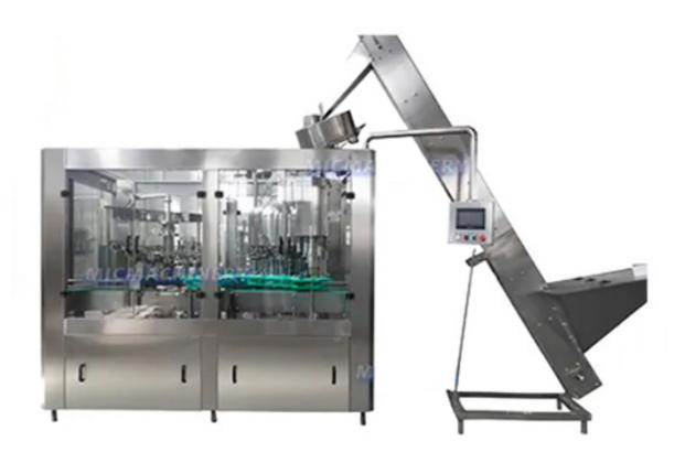
MIC 12-12-1 Juice Glass Bottle Filling Machine is applicable for juice glass bottle filling machine for mango juice, litchi juice, orange juice, apple juice and other Fruit and vegetable juice etc. (if need hot filling temperature at 85-90 degree)
