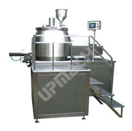
Rapid mixer granulator is also called high shear mixer granulator or wet granulator. It's an equipment that is used to mix powder ingredients and make granules. Rapid mixer granulator consists of mixing bowl, impeller, chopper, discharge port, liquid binder inlet port, pneumatic system and control system etc. This machine is widely used in pharmaceutical, foodstuff, chemical industry and light industry.
