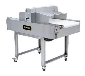
For quick and precise slicing in horizontal way, ANKO's Automatic Horizontal Cake Slicer is ideal for slicing various shapes of cake ranging from circle, rectangle, roll, triangle, etc. Double blades with vibration ensure every portion has a flat surface and pleasing look. It is an easy-to-operate and high quality machine.
