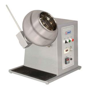
The Coating pan is used to produce uniform coating on tablets with the help of Baffles inside of pan. This can be mounting on the universal gearing and as a result different tilting angle can be set up to 45 Degree.
