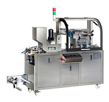
This blister Packaging machine is special designed for dosage room of hospital, middle or small pharmaceutical and nutrition products factory. It has features with small machine-body, flat structure mold.
