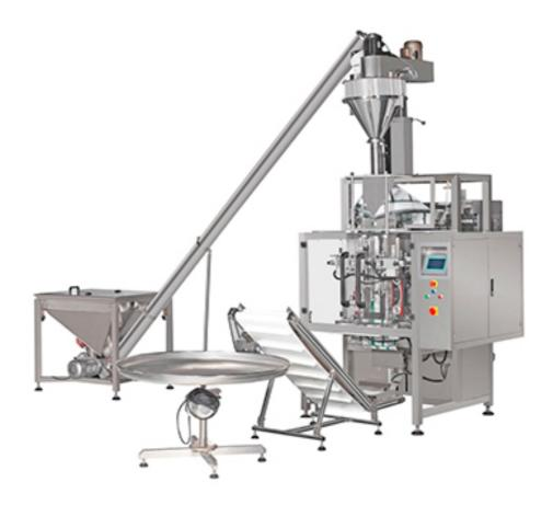
The packing machine is suitable to packaging powder, such as milk powder, coffee powder, tea powder, tea powder, face mark powder, spices, sweet flour, flour, etc
