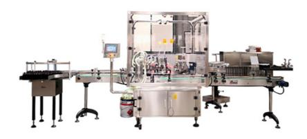
The machine is an auto-liquid filling devise which is composed of PLC, human-computer interface, and optoelectronic sensor and air-powered. Combined with filling, plugging, capping and screwing in one unit. It has the advantages of high accuracy, stable performance and greater versatility under extreme operating conditions which enjoys a high prestige. It has been widely applied in areas of pharmaceuticals industry.
