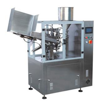
This machine fill and seal ointment, cream jellies, toothpaste, lotion, jam and viscosity material, sealing or tail folding, batch number embossing (include manufacture date) automatically. It's ideal equipment for aluminum tube, plastic tube and laminated tube.
