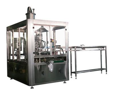
Automatic spout pouch pack filling and capping machine is suit for filling and capping liquid products, like juice, hand washing, etc, into stand-up pouch.
