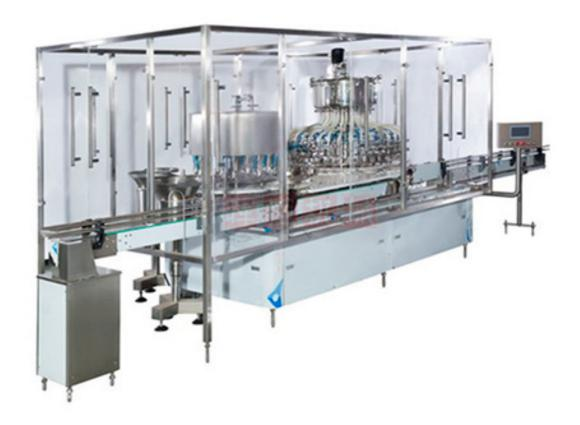
The glass infusion bottle enters the filling part in the way of fixed distance and bottle separation after passing the bottle feeding track and twisting into the bottle. The filling is measured by the principle of time and constant current. The filling amount is set and adjusted by the touch screen, and the measurement is stable and accurate.
