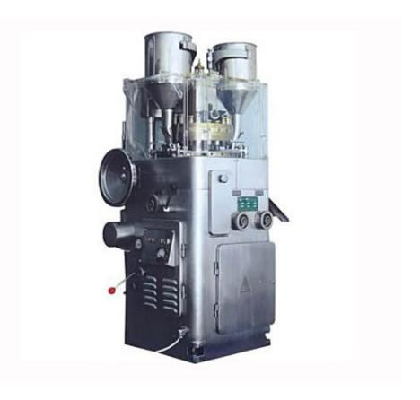
ZPW21A and ZPW21B rotary tablet presses are high speed rotary tablet machines. They are designed to meet the GMP standard. ZPW21B is the improved version of ZPW21A. It can be used for pressing tablets from various kinds of granular materials. It can press not only round tablets but also tablets in different geometrical shapes, double-layer and annular tablets. The tablets may have letters on both sides.
