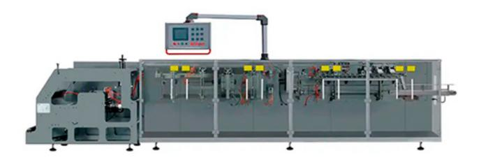
BHD-180SZ is specially designed for doypack bags with zippers. The maximum capacity of the bag is 1000ml. It is often used to package sugar, biscuits, match powder, chili powder and other powders or granules. The zipper function can also be added according to customer needs. Hanging holes and other functions provide a wider range of applications.
