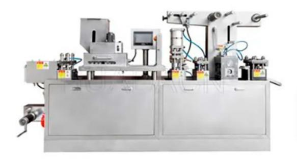
The product is specially designed for hospital dosage room, laboratory institute, health care product, middle-small pharmacy factory, and featured by compact machine body, easy operation, multi-function, stroke adjustable, long durability etc, it is suitable for the Alu-PVC package of medicine, food, electric parts etc.
