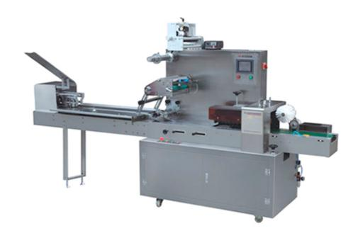
Flow Pack Machine – GZB model design provides for packaging of piece products in 3- side bags.
