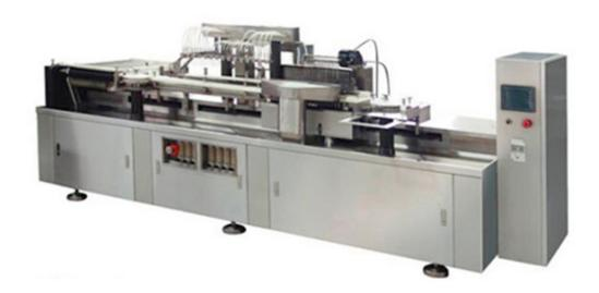
The machine is mainly used for filling and sealing ampoules in cleaning conditions in pharmacy factories.
