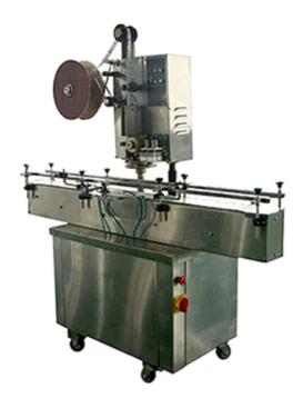
DI-200 is economical and easy to operate. The machine can automatically cut off the belted desiccant and insert it into the container accurately and speedy. This fully automatic machine inserts a predetermined length of desiccant coil into containers at speeds up to 80 cpm.
