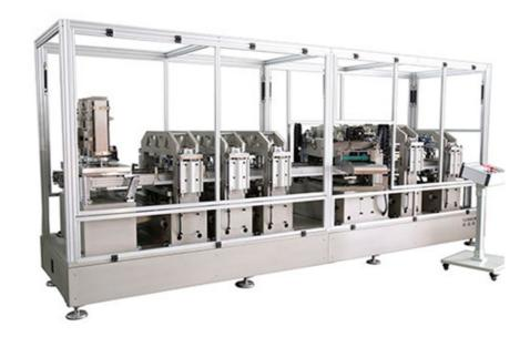
This machine can be used to manufacture 202-603# easy-tear lid, and especially suitable for bigger 307-603# iron easy-tear lid, It can automatically complete the functions of cover feeding, punching, deep drawing, crimping, aluminum foil pre-sealing, sealing, embossing and output etc. Independent servo controls each function module, adjusts parameters separately, and achieves high-speed response and synchronous movement. Inclined punching arrangement makes the aluminum foil waste least.
