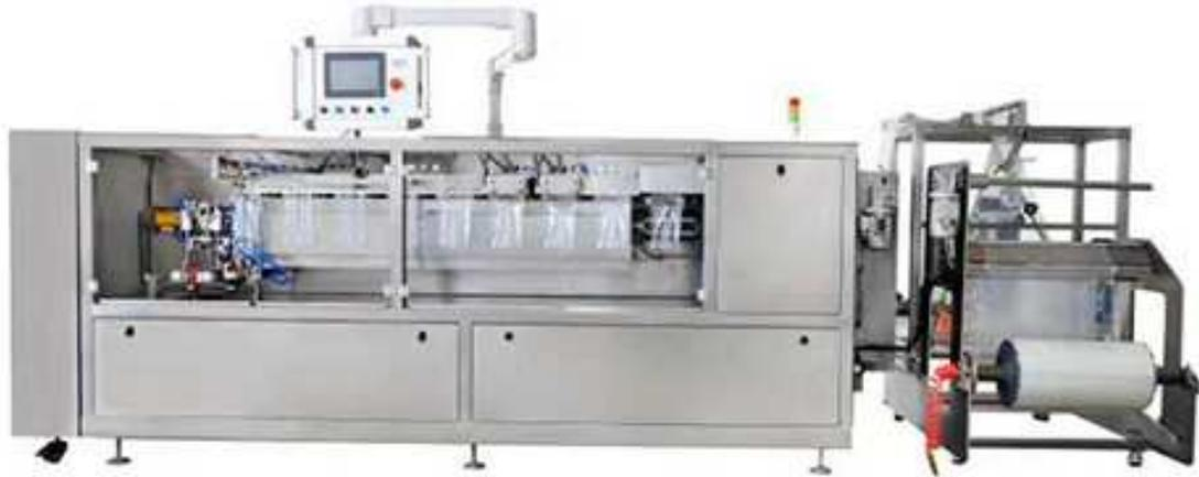
HD-300 Series designed for bigger volume doypack, with functions of making hanging hole, special shape, zipper or spout.
