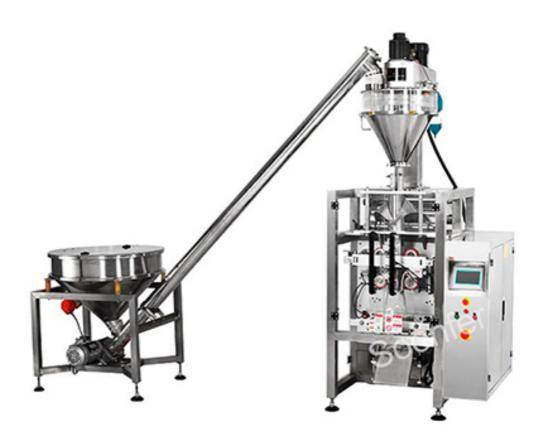
Automatic powder packing machine can making various bag shape such as pillow bag, gusset bag, pouching whole, link bag, quod seal bag etc. Imported servo motors film pulling system and with electric eye sensor control make more accuracy and well performance to make perfect bag shape.
