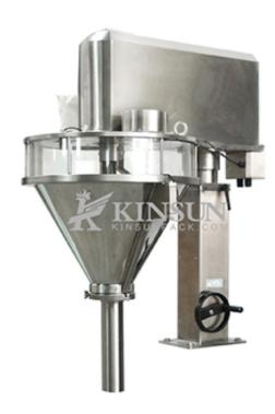
This type can do dosing and filling work. Due to the special professional design, it is suitable for the fluidic or low-fluidity materials, like milk powder, Albumen powder, rice powder, coffee powder, solid drink, condiment, white sugar, dextrose, food additive, fodder, pharmaceuticals, agriculture pesticide, and so on.
