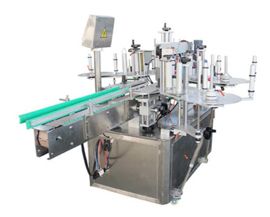
Dedicated to the circumferential surface of red wine bottle label, can be attached to a single standard and double standard, are back double standard spacing can be flexibly adjusted; possess conical bottle labeling function; optional peripheral location detection device can achieve the specified position in the circumferential surface labeling.
