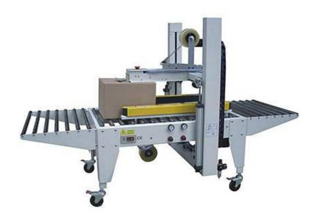
Automatic carton sealer adopts two motor driving, top and bottom sealing. Automatically adjust the height and the width for different size of cartons, suit for pack different cartons at the same time.
